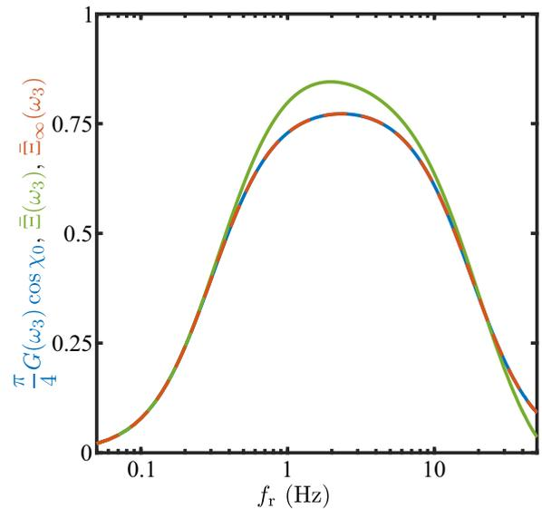
FIG. 22. Response functions. For  $\kappa = \tau_d = 0$ , the graph compares the steady-state response function  $(\pi/4)G(\omega_3) \cos \chi_0$  in Eq. (31) (dashed blue), the initial average response  $\bar{\Xi}(\omega_3)$  in Eq. (A9) (green) and the  $n \rightarrow \infty$  limit of the transient response  $\bar{\Xi}_\infty(\omega_3)$  (dashed red), as functions of  $f_r = \omega_3/2\pi$ .
