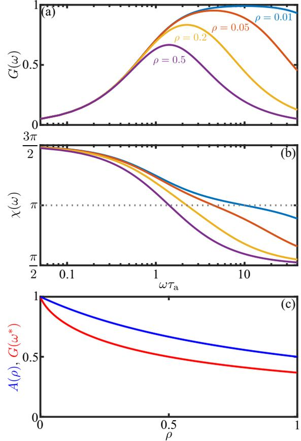
FIG. 13. Dynamics of the adaptive model. (a) Gain (31a) for various values of  $\rho = \tau_r/\tau_a$ . (b) As in panel (a), but for the phase shift  $\chi$  (31b), with  $\tau_d = 0$ . (c) Comparison of peak amplitude for step-up and oscillatory forcing as a function of  $\rho$ .
