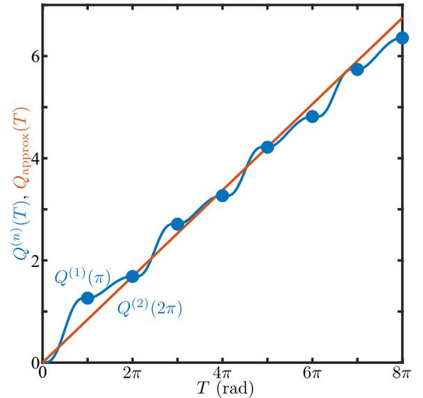
FIG. 23. The functions  $Q(T)$ . The function  $Q^{(n)}(T)$  (blue), defined in a piecewise manner between endpoints (blue circles), can be approximated as a straight line  $Q_{\text{approx}}(T) = \bar{\mathcal{Q}}T$  (red). Both  $Q^{(n)}(T)$  and  $\bar{\mathcal{Q}}$  were computed with the experimentally derived  $\tau_r = 0.009$  s and  $\tau_a = 0.524$  s. The value of  $f_r$  was taken to be 1.67 Hz. The value of  $\bar{\mathcal{Q}}(\omega_3, \tau_r, \tau_a)$  was calculated to be 0.268.
