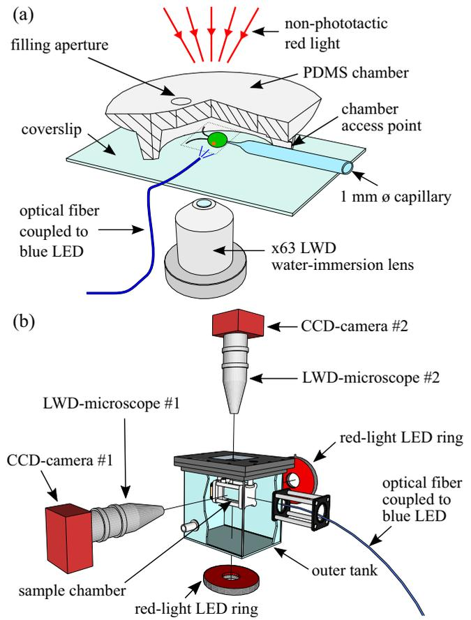
FIG. 3. Experimental methods. Setups to measure (a) the flagellar photoresponse of cells immobilized on a micropipette, and (b) swimming trajectories of phototactic cells in a sample chamber immersed in an outer water tank to minimize thermal convection, as described in text.
