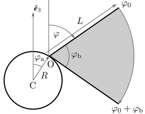
FIG. 8. The pivoting-rod model of the power stroke.
